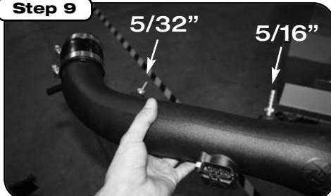
Step 9 Install MAF sensor to new tube using M4 screws, spacers and gasket provided. Make sure spacers and gasket are between sensor and tube. Install brass nipples to tube and tighten.
