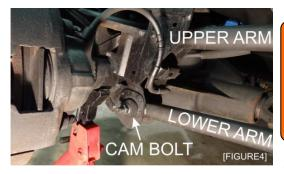
and re-use the cam bolt, place a line on the washer and frame with chalk or marker to indicate the position of the cam bolt for reinstallation later. Remove the front cam bolt. Remove rear mounting bolt. This will release the lower arm completely.
