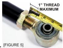
**<u>UNDER NO CIRCUMSTANCES</u>** should the arms be adjusted beyond the point where more than 1" of joint threads are exposed! Extending the arms further can lead to critical failure that could result in vehicle damage, personal injury, and even death. Any adjustment beyond 1" of exposed threads will void all warranties.
