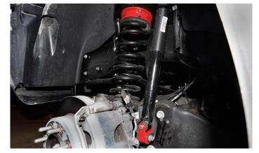
**9.** Re-install the tires and lower the axle. Raise the frame to remove the jack stands. Lower the frame such that the full weight of the vehicle is on the suspension. Tighten the lock nut on the the upper shock stem until it bottoms out and torque to setting specified in the vehicle owner's manual.
