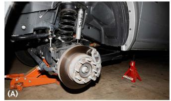
**2.** Repeat each step of installation on both sides of the vehicle at the same time. Remove the bolts from the lower shock mounts on the axle. Using the floor jack, move the axle up or down to set the axle right at the end of the shock travel. This makes removing the shock bolts easier.
