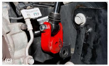
**5.** Install the HBS spacer onto the upper coil spring mount with the provided 12MM fastener (**figure D**). Torque to spec.
