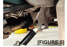
Install the rear joint first using the new HBS-
