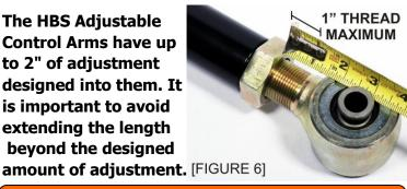
**UNDER NO CIRCUMSTANCES** should the arms be adjusted beyond the point where more than 1" of joint threads are exposed! Extending the arms further can lead to critical failure that could result in vehicle damage, personal injury, and even death. Any adjustment beyond 1" of exposed threads will void all warranties.
