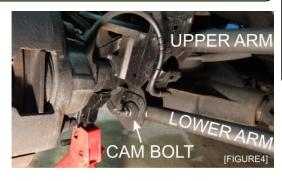
Remove the front OEM cam bolt. Remove rear mounting bolt. This will release the lower arm completely.
