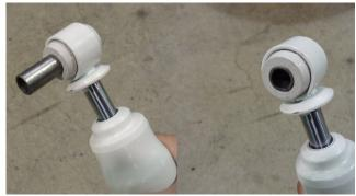
6. Attach the cylinder end of the stabilizer shock to the Center Bracket. Install the 12mm carriage bolt through the cylinder end of the stabilizer shock. Continue to install through HBS Center Mount Bracket, the 10mm-thick spacer, lock-washer and nut, as shown in the figure below. Torque 12mm bolt to 72 ft/lbs.
