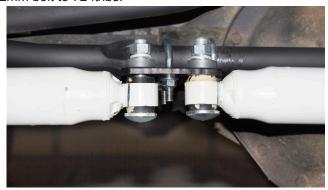
**7.Attach the rod end of the shock to the HBS Side Bracket.** Place the 12mm hex bolt and flat washer through the shock and side bracket, as shown in the figure below.
