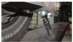
Drill the outside mounting hole and install the bolt, washer, and nut.
