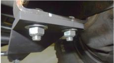
Torque the nuts to 26 ft/lbs. Repeat on driver's-side.
