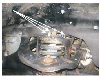
5. Remove the strut assembly from the vehicle and mount it in a bench vise. Install the Hell Bent Steel strut extension on the top of the strut assembly.
