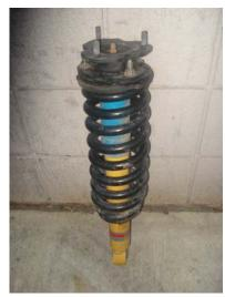
**6.** Run down nuts snug with end wrench. Torque to OEM specs.
