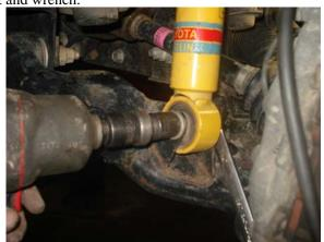
NOTE: Once the nut is removed, it may be necessary to use a punch and hammer to free the bolt.
