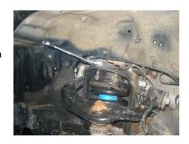
**8.** Use a pry bar to position the lower control arm and the strut mount, and then reinstall the mounting bolt. Torque to OEM specs. HINT: It may be helpful to use a pry bar to press down on the steering knuckle for reinstalling the mounting bolt.
