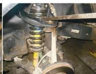
**9.** Place a jack under the lower control arm. Raise the lower control arm to reattach the lower ball joint bolts. Torque the ball joint nuts to OEM specs.
