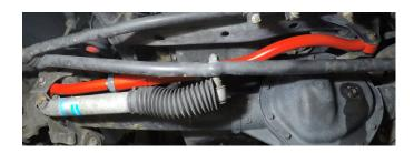
8. There is no perfect length for your Hell Bent Steel Trackbar. To determine the setting that will work best for you, start by setting the axle as close to the center of the vehicle as possible. Tighten the jam nuts and take the vehicle for a test drive. On your test drive make sure to turn the wheel to its furthest extents and watch for any rubbing or collision issues.
