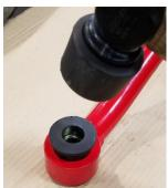
4. To install the bushings, set one bushing on a table and use a rubber mallet to install the sleeve into the middle of the bushing.
