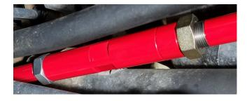
7. Adjusting the Hell Bent Steel Trackbar can be done while the bar is installed on your vehicle. Spin the center link to adjust the length of the bar as needed.
