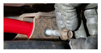
6. Install the bar into the lower mount first. The new bar will be a tight fit, you may need to wiggle the bar while pushing it into the mount. Place the lower bolt through the hole. Install the bar into the upper mount. Once both bolts are in, install the nuts and torque the fasteners to 126 ft-lbs
