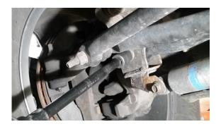
2. Remove the Trackbar and set aside. Retain the bolts and nuts for reuse.
