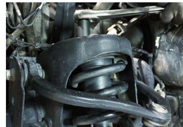
**2.** Remove the upper strut mount nuts with a 15mm wrench or socket. You will need a socket to remove the far strut mount.
