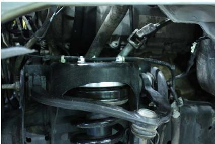
11. Place strut back into upper strut mount. Snug provided nuts with wrench or ratchet (after install, you will torque to OEM specs).
