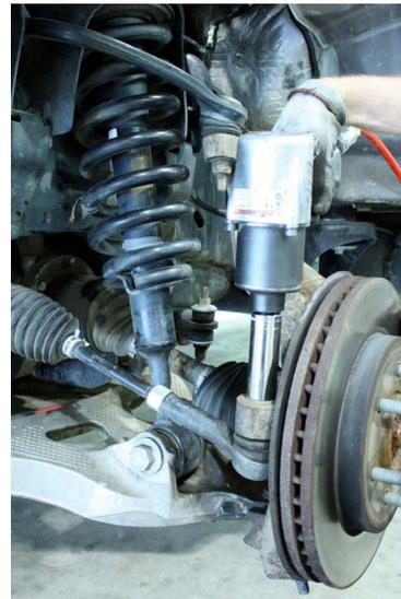
**4.** Disconnect the tie rod end with a 21mm socket. Using a ball peen hammer or impact tool, hit the steering knuckle (not the tie rod) until the tie rod pops out.
