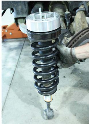
9. Place the Hell Bent Steel strut extension on the top of the strut.
