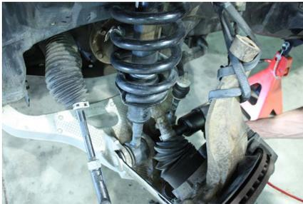
7. Next remove the strut's lower bolt. Using a 27 mm wrench, hold the nut and remove the bolt with a 30 mm socket.
