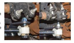
**8. Position the HBS Center Mount Bracket.** With your wheels straight, measure the length of exposed rod of each of the stabilizer shocks. Adjust the HBS Center Mount Bracket until there is equal extension of both shocks. Once the bracket is centered, tighten U-bolts and torque to 26 ft-lbs.
