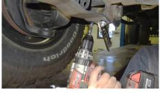
Make sure that the rear-facing edges of the HBS Bracket and the lower control arm bracket are aligned and tighten both nuts.
