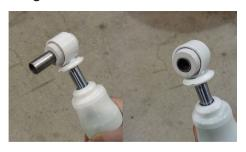
6. Attach the cylinder end of the stabilizer shock to the Center Bracket.
