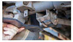
Using the drill and 25/64 bit, drill through the inside mounting hole, using the HBS Bracket as a guide.
