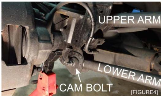
Remove the front OEM cam bolt. Remove rear mounting bolt. This will release the lower arm completely.
