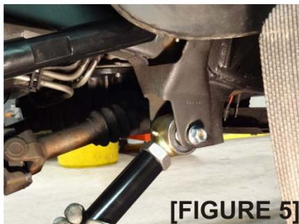
Install the rear joint first using the new HBS-provided **16mm** hardware with the washer on the bolt head and the nut toward the outside of the vehicle. Next install front cam bolt (align with the mark made in Step 3) or the HBS Cam Bolt Eliminator Kit. Place the nut toward the outside of the vehicle.
