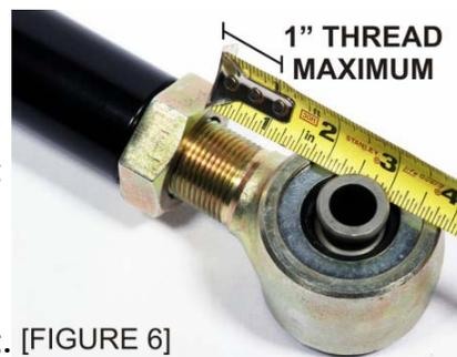
**UNDER NO CIRCUMSTANCES** should the arms be adjusted beyond the point where more than 1" of joint threads are exposed! Extending the arms further can lead to critical failure that could result in vehicle damage, personal injury, and even death. Any adjustment beyond 1" of exposed threads will void all warranties.
