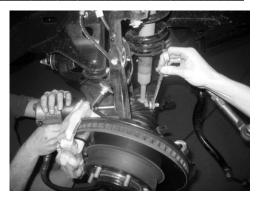
9. Remove the strut assembly from the vehicle and mount it in a bench vise. Install the Hell Bent Steel strut extension on the top of the strut, hold the part up to start the factory nuts onto the factory studs.
