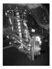
2. Using a 17mm ratchet, remove the nut from the bolt connecting the front sway bar link and the steering knuckle on both sides of the vehicle.
