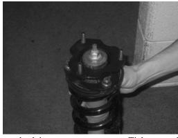
11. Place strut back into upper strut mount. Tighten provided nuts snug with wrench or ratchet (after install, you will torque to OEM specs).
