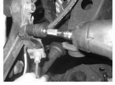
4. Detach all brake hose brackets from the steering knuckle and upper control arm. On vehicles with ABS, remove the front wheel speed sensor-retaining bolt and detach the sensor from the steering knuckle.
