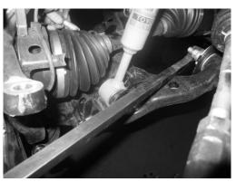
**13.** Place a jack under the lower control arm. Raise the lower control arm to reattach the lower ball joint bolts. Torque the ball joint nuts to OEM specs.
