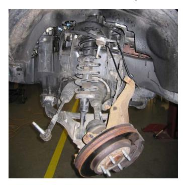
**7.** Next remove the struts lower bolt. Using a 27 mm wrench, hold the nut and remove the bolt with a 30 mm socket.
