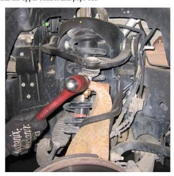
**6.** Support the knuckle with a bungee cord or safety wire so not to overextend the CV axel or stretch the brake hydraulic hose.
