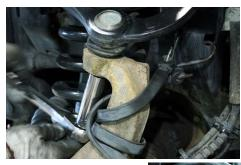
**5.** Support the knuckle with a bungee cord or safety wire so not to overextend the CV axle or stretch the brake hydraulic hose.
