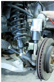
If you use a tierod pickle fork, be careful not to cut the tie rod boot. A severed tie rod boot will allow dirt and moisture to damage the tie rod end.
