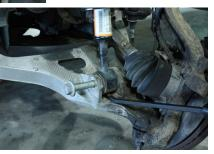
**13.** Place a jack under the lower control arm. Raise the lower control arm to reattach the ball joint. A pry bar may be used to hold the upper control arm into position. Torque the ball joint nut to OEM specs.
