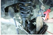
9. Place the Hell Bent Steel strut extension on the top of the strut.
