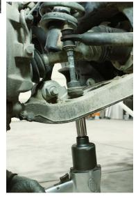
**4.** Disconnect the tie rod end with a 21mm socket. Using a ball peen hammer or impact tool, hit the steering knuckle (not the tie rod) until the tie rod pops out.
