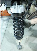
**11.** Place strut back into upper strut mount. Snug provided nuts with wrench or ratchet (after install, you will torque to OEM specs).
