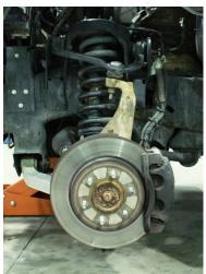
**2.** Remove the upper strut mount nuts with a 15mm wrench or socket. You will need a socket to remove the far strut mount.
