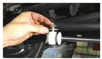
Tighten the bolt/nut and torque to 72 ft-lbs. Repeat on opposite side.
