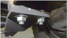
Torque the nuts to 26 ft/lbs. Repeat on driver's-side.
