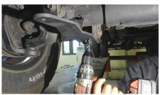
Leaving the clamp in place, insert one of the 3/8" X 1" bolts through the top. Secure with flat washer and nut.
