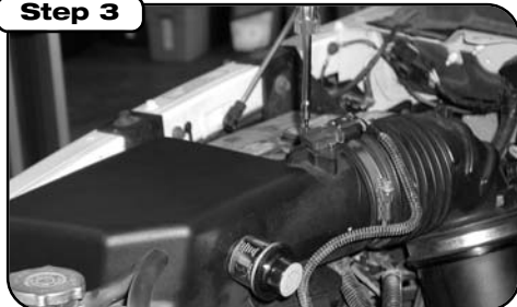
Disconnect the factory wiring harness from the intake temperature sensor located on the top of the airbox. Remove the intake temperature sensor from the airbox and set aside.
