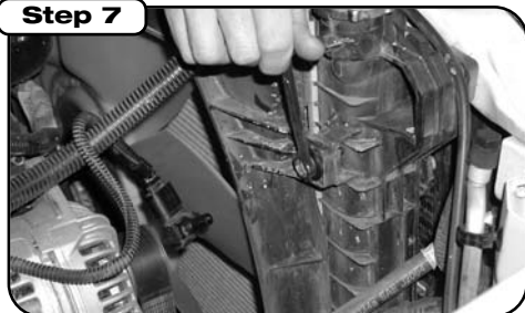
Using a 13mm wrench, loosen and remove the upper passenger-side bolt on the radiator shroud and set aside for installation of heat shield. Verify that the engine is cool, then temporarily remove the overflow hose from the radiator filler neck for clearance.
