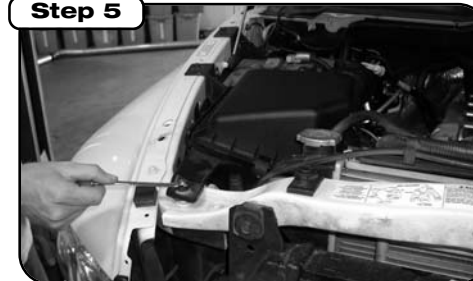
Using 10 mm wrench, remove the bolt that secures the factory airbox to the radiator bulkhead.
