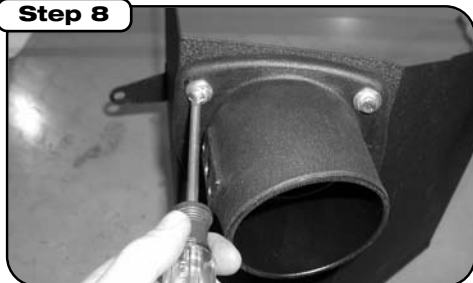
Install aFe intake tube and trim seal on the heat shield, be sure to install in the orientation shown. Install heat shield into engine compartment but do not attach any bolts. The bottom louvered panel must be positioned above the aluminum A/C line.
