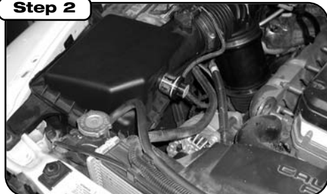
Complete stock intake. Make sure that the engine has sufficiently cooled down prior to starting installation of this kit.
