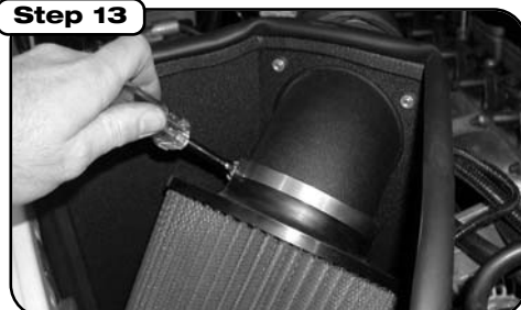
Install pre-oiled filter onto intake tube and tighten. Do not use any oil or grease when attaching filter. Reattach radiator overflow hose that was removed in Step 7.
