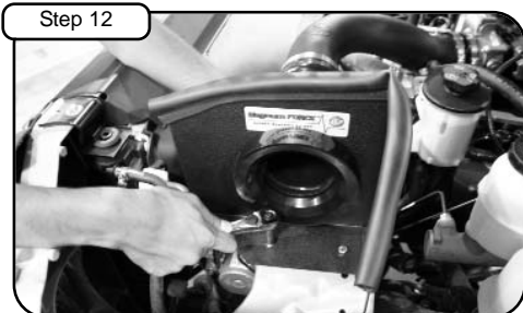
Tighten housing using 11mm socket or wrench. Install 3/4" trim seal to housing.
