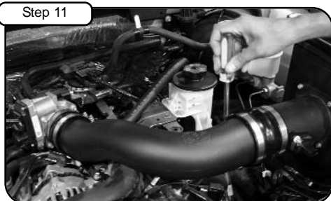
Install new tube to throttle body and intake housing. Tighten clamps with 5/16" nut driver. Finish install on crank case line with mini clamp and tighten.
