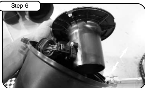
Disconnect band clamp and with flat head screwdriver, disconnect other end of MAF harness. Carefully pull out OE MAF sensor tube.
