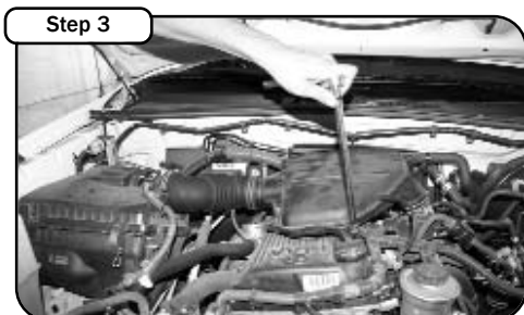
Step 3 Remove the three bolts that secure the intake resonator to the valve cover. Loosen the intake hose clamps.
