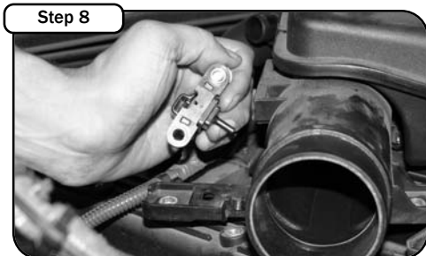
Step 8 Remove the VSV located on the back side of the intake resonator. Remove intake resonator.
