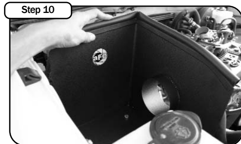
Step 10 Install 3/4" trim seal to housing. Secure the housing to the engine compartment with M8 screws and washers provided.
