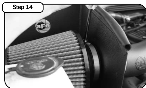
Step 14 Install air filter into housing and tighten using 5/16" nut driver.
