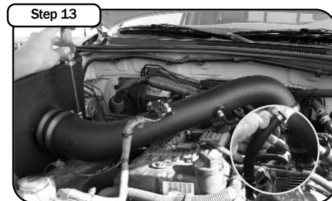
Step 13 Install crank case hose with mini clamps provided and tighten to tube. Tighten all clamps. Reconnect the MAF sensor harness.
