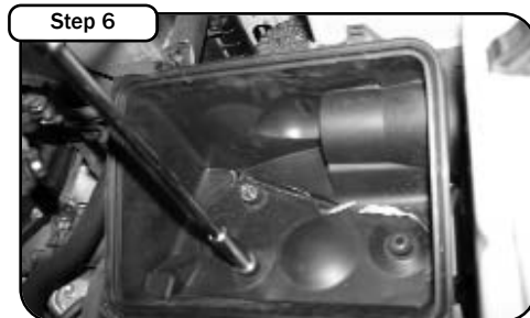
Step 6 Remove the three 12mm bolts securing the lower air box. Remove the bolt securing the windshield washer reservoir. Remove the lower air box.
